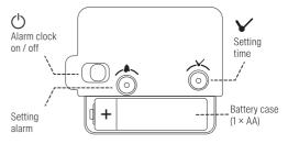
The alarm clock function can be de-/activated at the on/off switch.
